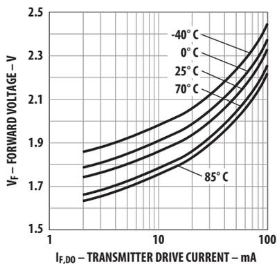
Figure 1. Typical forward voltage vs. drive current
