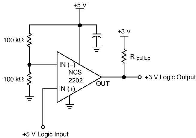
This circuit converts 5 V logic to 3 V logic. Using the NCS2202/A allows for full 5 V logic swing without creating overvoltage on the 3 V logic input.
