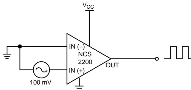
**Figure 21. Zero-Crossing Detector**
