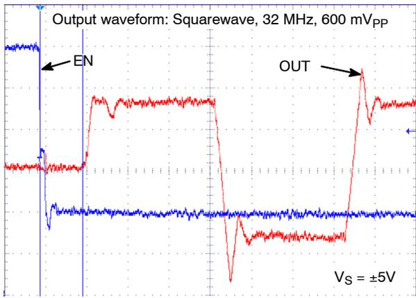
**Figure 23. Turn ON Time Delay**
