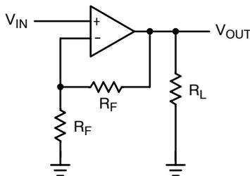
**Figure 4. Typical Test Setup**
