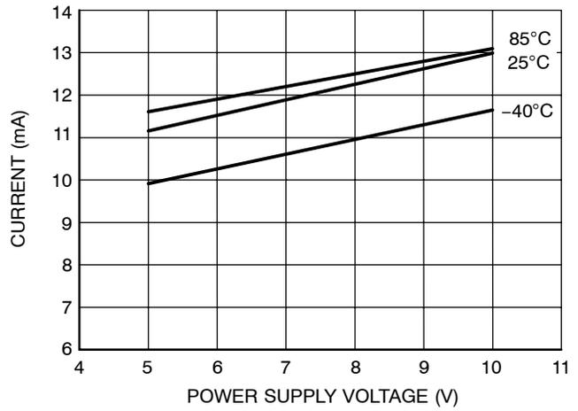
Figure 18. Supply Current vs. Power Supply Voltage (Enabled)
