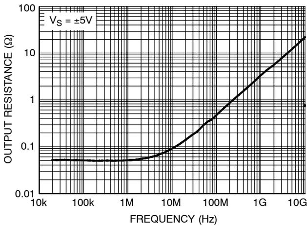
Figure 21. Closed Loop Output Resistance vs. Frequency
