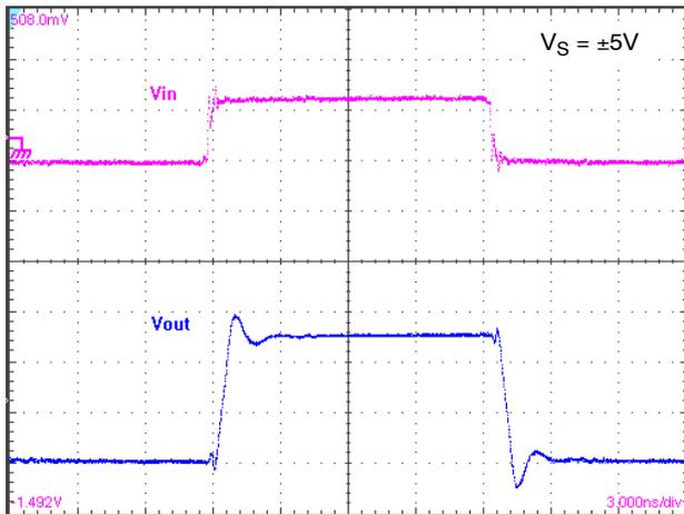
Figure 9. Small Signal Step Response
