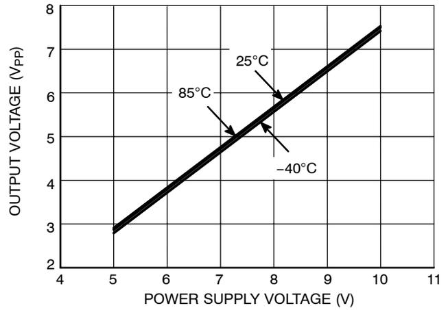
Figure 20. Output Voltage Swing vs. Supply Voltage
