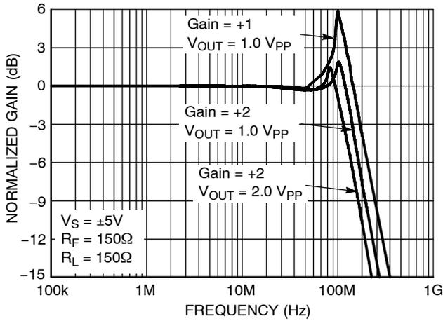
Figure 7. Large Signal Frequency Response
