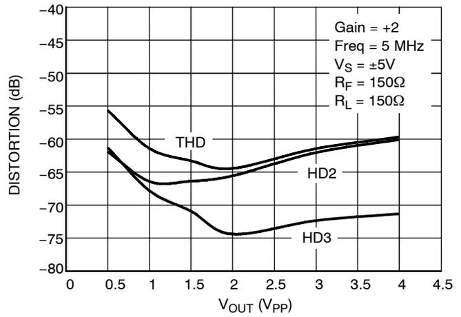
Figure 12. THD, HD2, HD3 vs. Output Voltage
