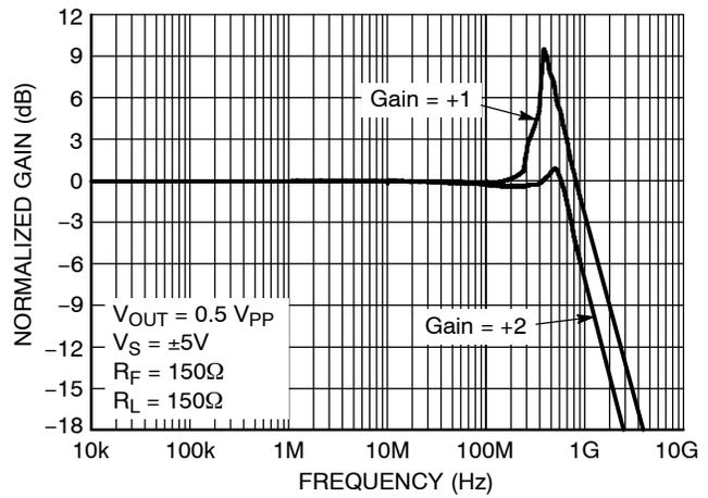
Figure 8. Small Signal Frequency Response
