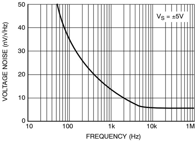
Figure 13. Input Referred Voltage Noise vs. Frequency
