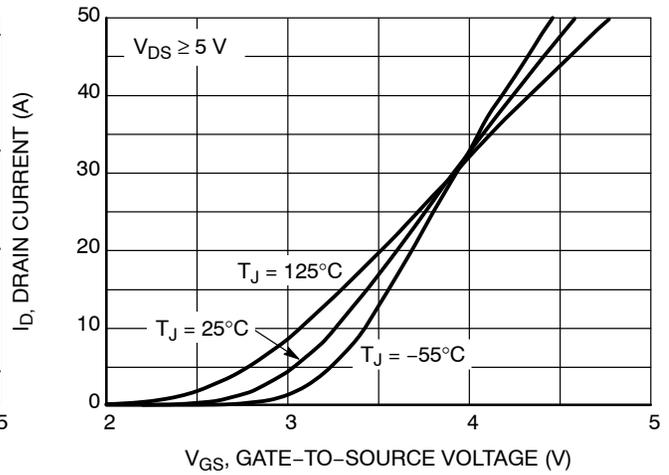
Figure 2. Transfer Characteristics
