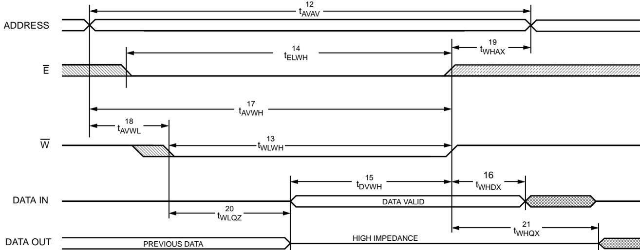
SRAM WRITE CYCLE #2:  $\bar{E}$  Controlled<sup>j</sup>
