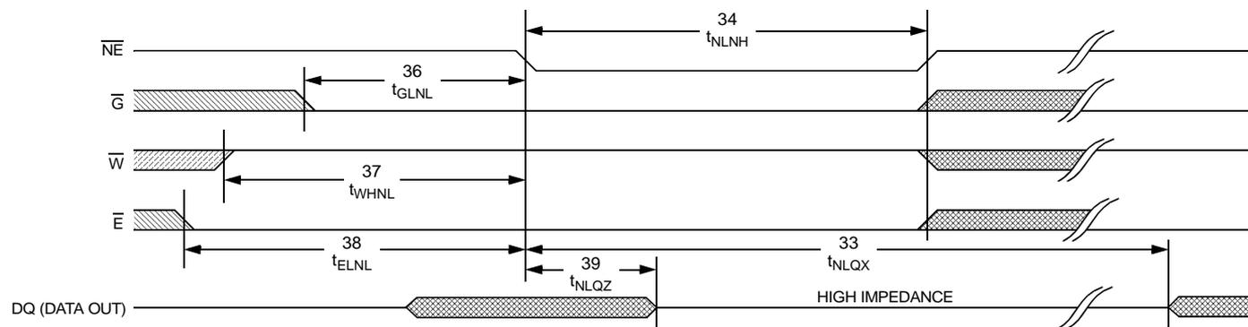
RECALL CYCLE #2:  $\overline{E}$  Controlled<sup>o</sup>
