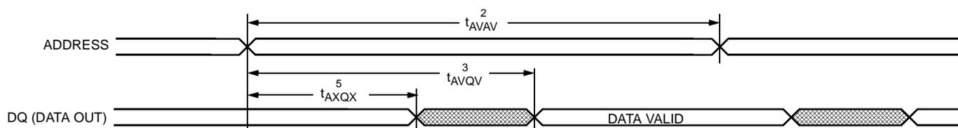
SRAM READ CYCLE #2:  $\overline{E}$  Controlled<sup>f</sup>
