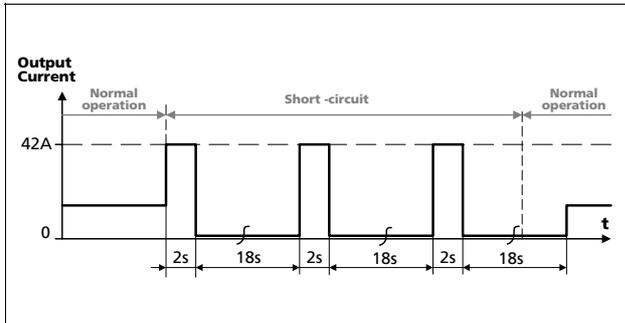
Fig. 6-4 **Dynamic overcurrent capability, typ.**
