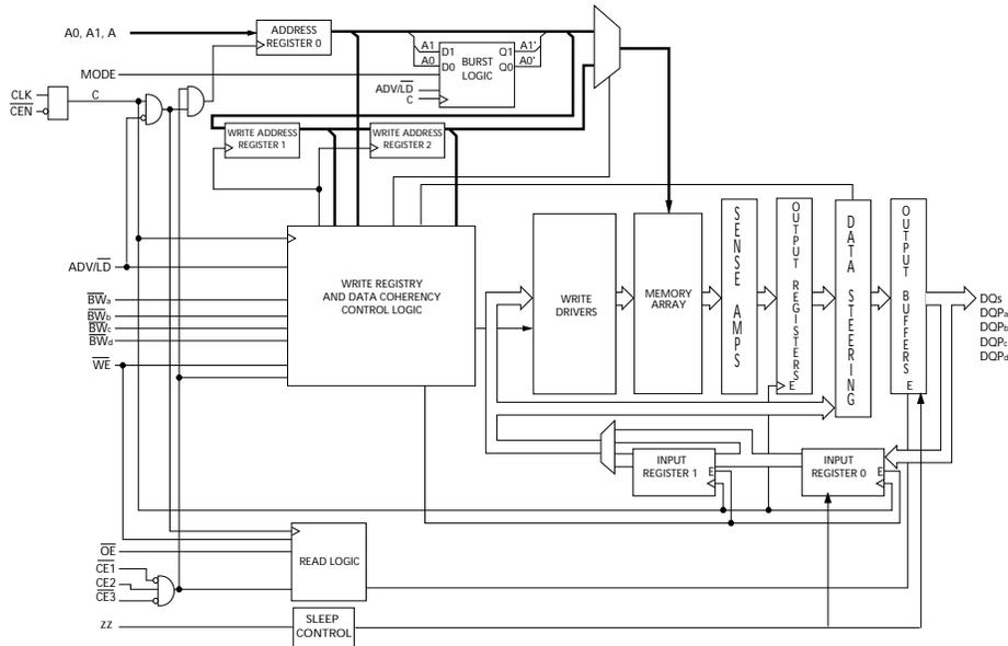
**Logic Block Diagram – CY7C1462KV25**
