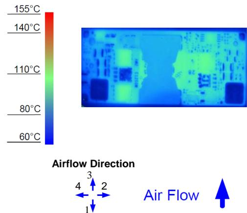
**Figure 8.** Thermal Image for Airflow Direction 3
