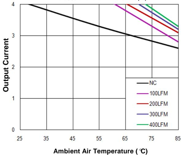
**Figure 7.** Current Derating Curve for Airflow Direction 3
