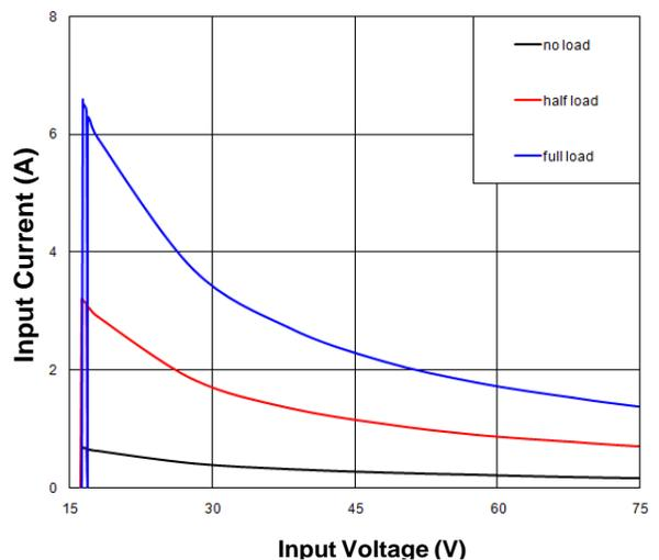
Figure 2. Input Characteristics
