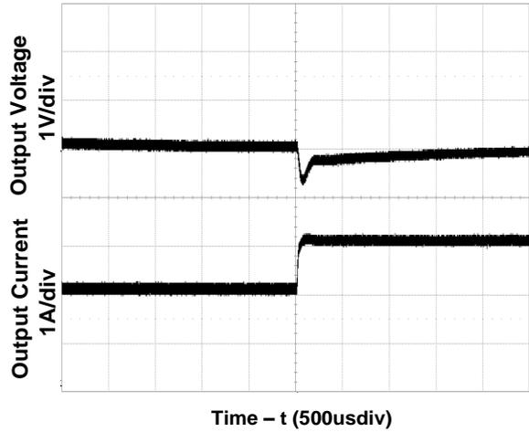
**Figure 6.** Transient Load Response
