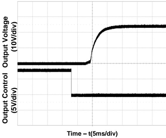
**Figure 3.** Start-Up from Enable Control
