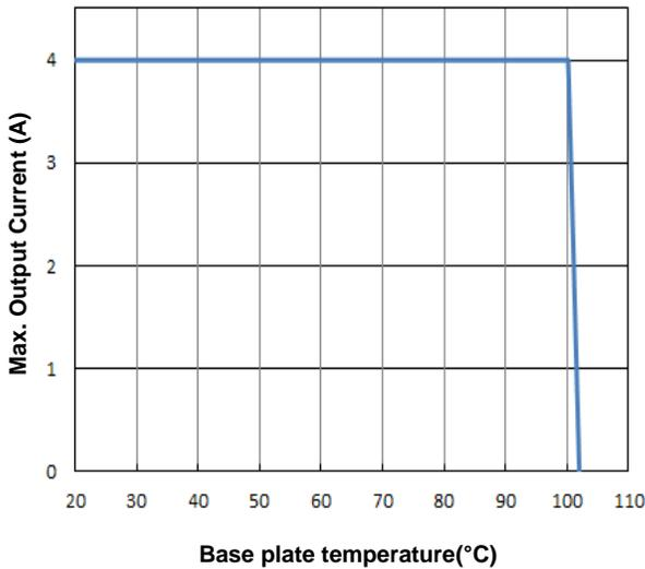
**Figure 9.** Current Derating Curve for Base plate
