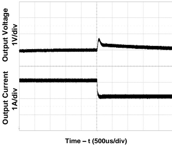
**Figure 5.** Transient Load Response
