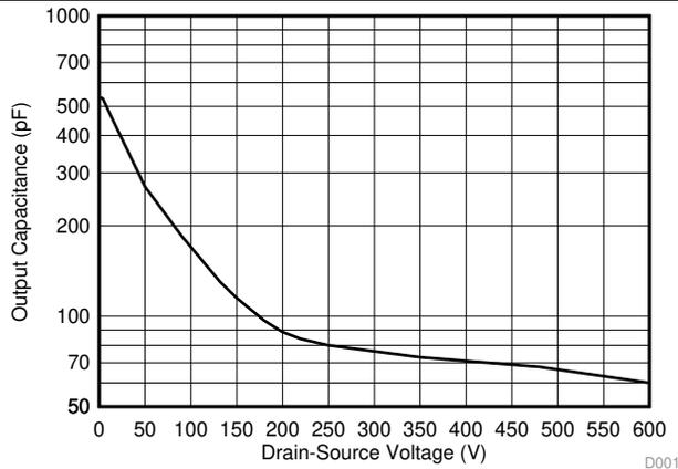
Figure 7. Output Capacitance
