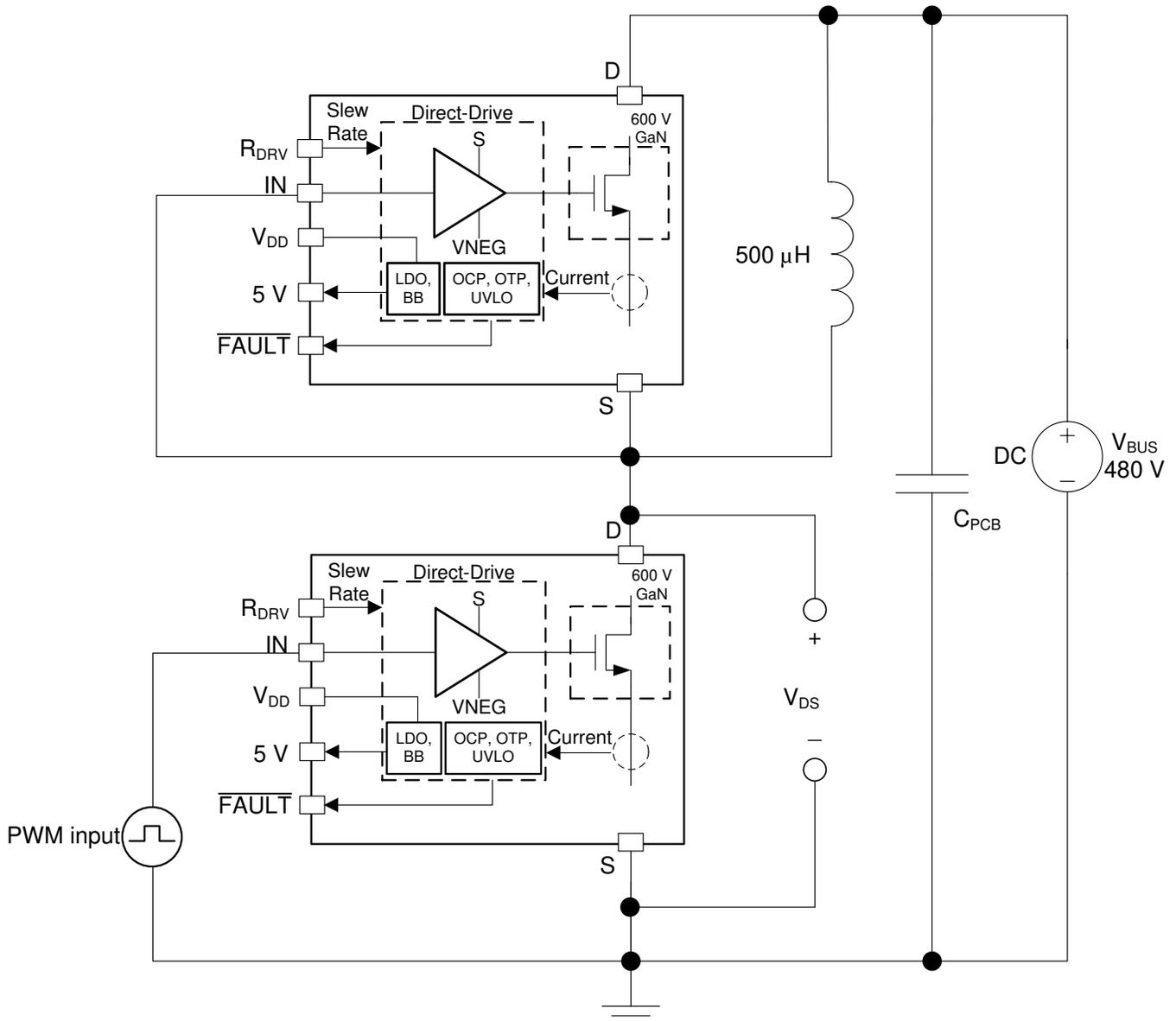
**Figure 11. Circuit Used to Determine Switching Parameters**
