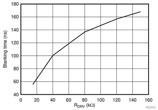
Figure 10. RDRV vs Blanking Time
