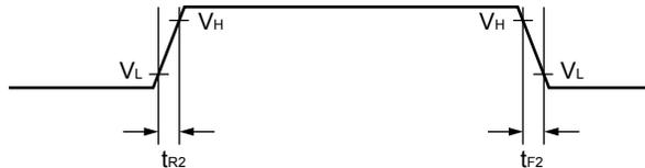
$$V_H = V_{OL2} + 0.1 \times (V_{OH2} - V_{OL2})$$
