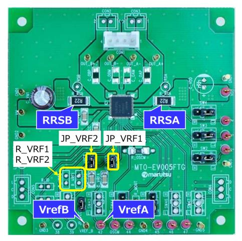
The TB67S261FTG conducts motor operation by PWM constant current control which is based on the frequency of the OSCM oscillation circuit. The maximum current value (set Motor current value) can be determined by a sense resistor (RRS) and the reference voltage (Vref).
