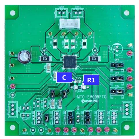
In PWM control of the TB67S261FTG, the internal oscillation frequency (fOSCM) and the chopping frequency (fchop) can be adjusted according to the constant of the external components those are connected to the OSCM pin. In general,  $f_{chop}$  is recommended to set in the frequency range of 40kHz to 150kHz.
