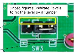
On this evaluation board, jumpers as shown in the picture above are provided for setting operation of TB67S261FTG
