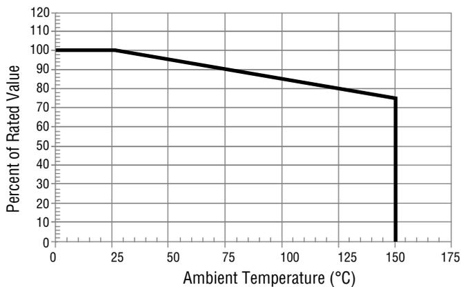
This graph shows the typical device surge current derating versus ambient temperature when subjected to the 8/20  $\mu s$  current waveform per the IEC 61000-4-5 specification. This device is not intended for continuous operation at temperatures above 125  $^{\circ}C$ .
