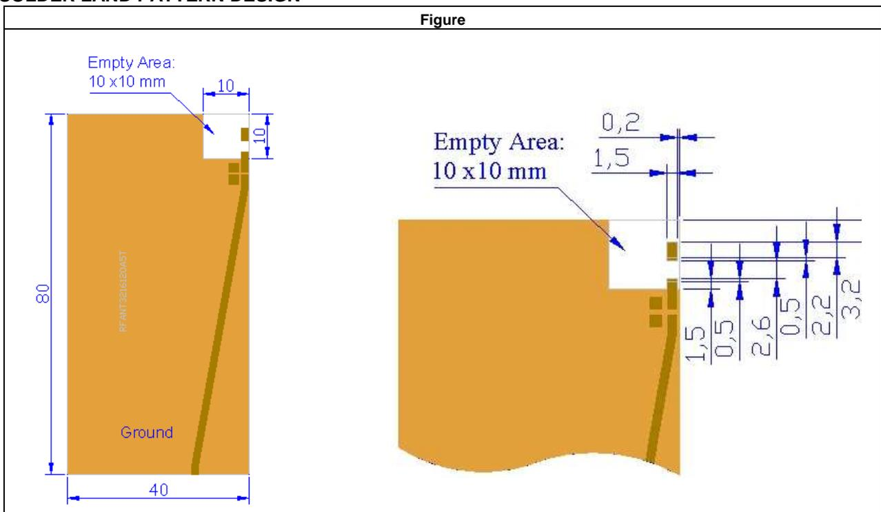
**Antenna on Test Board ( Thickness 0.8mm)**
