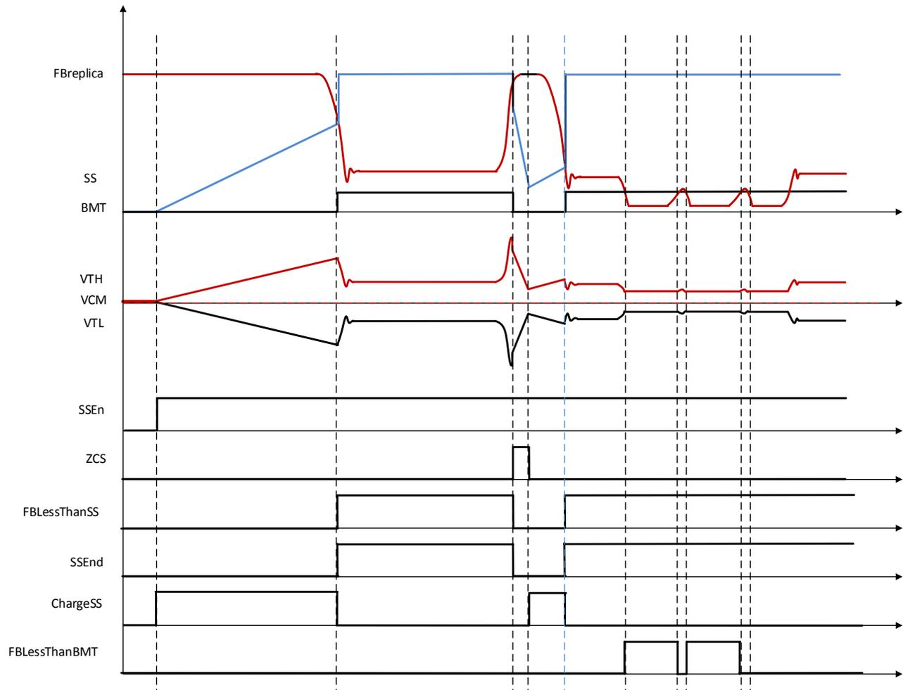
Figure 7-4. Feedback Chain Timing Diagram
