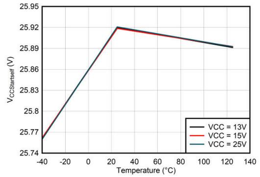
**Figure 6-24. V<sub>CCstartself</sub> vs Temperature**
