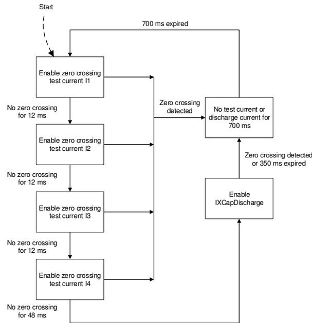
**Figure 7-16. AC ZCD and X-Capacitor Discharge Flow Chart**
