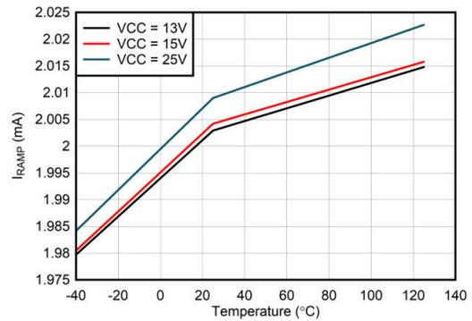
**Figure 6-6. I<sub>RAMP</sub> vs Temperature**
