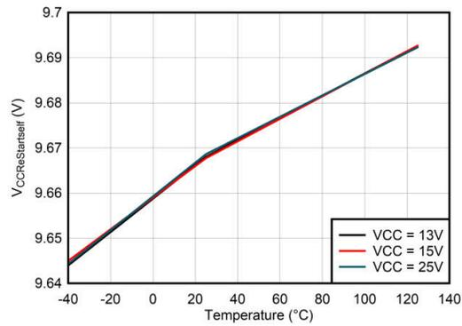
**Figure 6-25. V<sub>CCRestartJfet</sub> vs Temperature**
