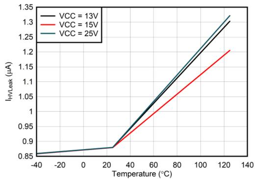
**Figure 6-3. I<sub>HVLeak</sub> vs Temperature**
