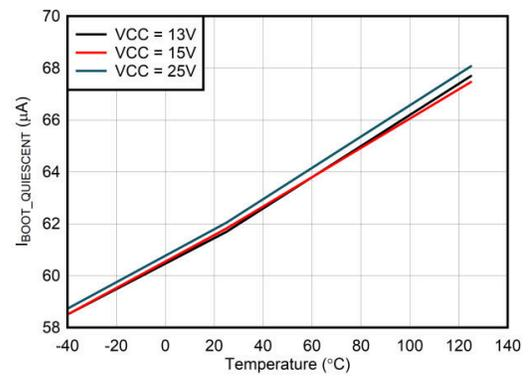
**Figure 6-4. I<sub>BOOT\_QUIESCENT</sub> vs Temperature**
