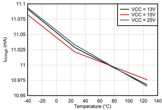
**Figure 6-1. I<sub>HVHigh</sub> vs Temperature**
