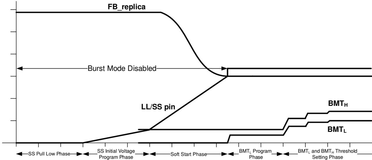
**Figure 7-20. Timing Diagram of LL/SS Pin Programming**
