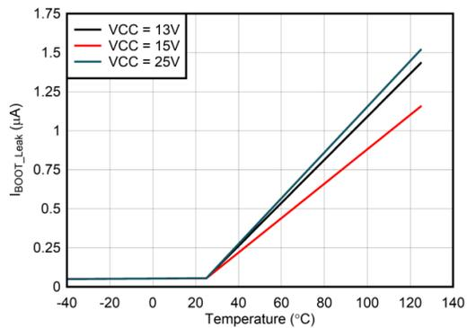
**Figure 6-5. I<sub>BOOT\_LEAK</sub> vs Temperature**
