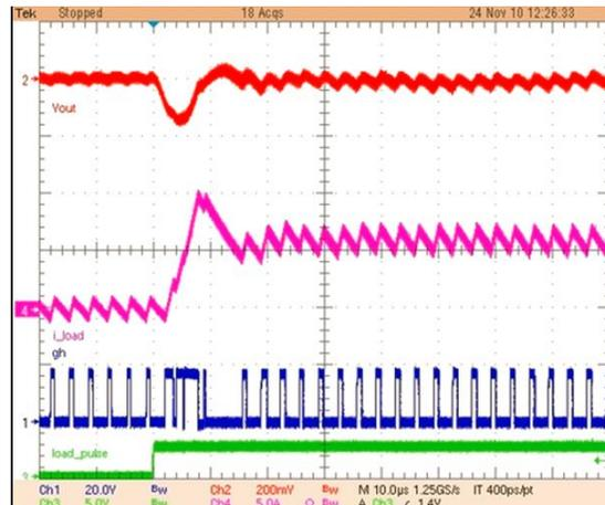
Fig. 8 10-6A Transient 300kHz with OVS  $\pm 5.5\%$
