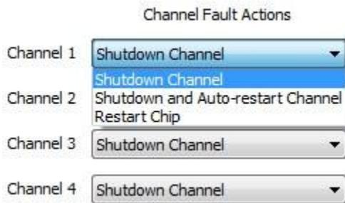
In the case of shutting down the faulting channel and auto-restarting, the user has an option to specify startup timeout (the time in which the fault is validated) and hiccup timeout (the period after which the controller will try to restart the channel) periods in 1 msec increments with a maximum value of 255 msec.
