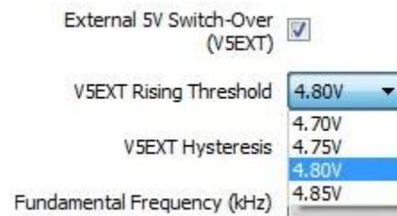
When the controller switches over to the V5EXT rail, the V5EXT\_RISE interrupt is generated to inform the host. Similarly, when the controller switches out, the V5EXT\_FALL interrupt gets generated.
