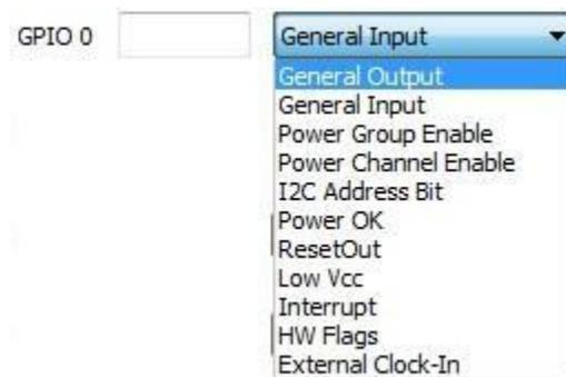
**HW Flags** – these are hardware monitoring functions forwarded to GPIO0 only. The functions include Under-Voltage Warning, Over- Temperature Warning, Over-Voltage Fault, Over-Current Fault and Over -Current Warning for every channel. Multiple selection is available in which case the resulting signal is the OR logic function
