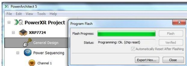
For users that wish to create their own programming procedure so they can re-program Flash in-circuit using their system software, please contact Exar for a list of I2C Flash Commands needed.
