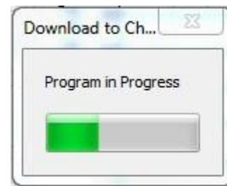
By clicking on the Flash button, user will start programming sequence of the design configuration into the Flash NVM. After the programming sequence completes, the chip will reset (if automatically reset After Flashing box is checked), and boot the design configuration from the Flash.
