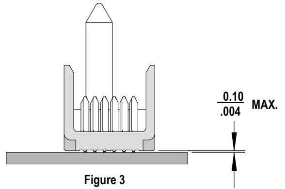
There should be no broken stand-offs along the perimeter of the part (an indication of over-pressing).
