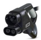
DC charging cable, DC charging cable with vehicle connector, open cable end, CCS type 2, Combined Charging System, IEC 62196-3, 125 A / 1000 V (DC), design line Standard, cable: 4 m, black, straight, mating face: black, handle area: gray
