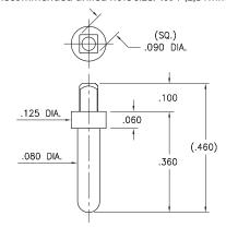
Recommended drilled hole sizes are prior to plating of the PCB and based on typical copper deposition of .5 - 1 oz. This results in a reduction of hole size by approximately .0015" - .003". Depending on surface plating, typical finished hole sizes are .003" - .005" smaller than drilled hole sizes. The finished hole size tolerance for press-fit applications should be specified as +/- .002"
