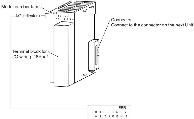
**Note:** The CJ1W-OD202, CJ1W-OD204, and CJ1W-OD212 also have an ERR indicator for the load short-circuit alarm.
