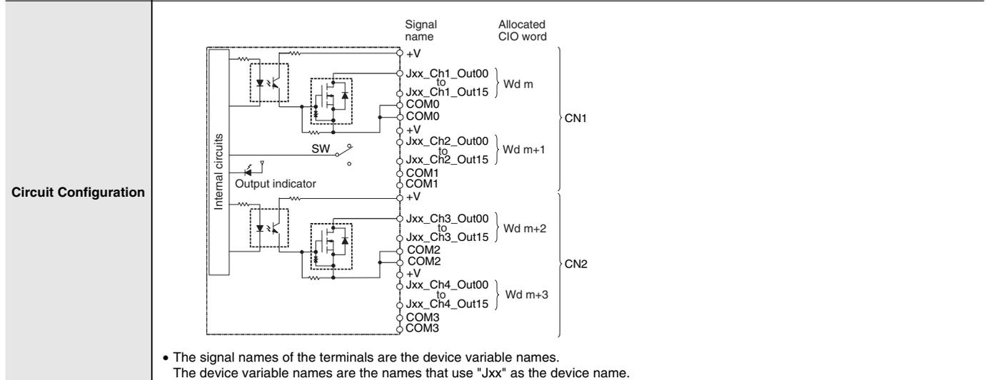
External connection and terminal-device variable diagram
