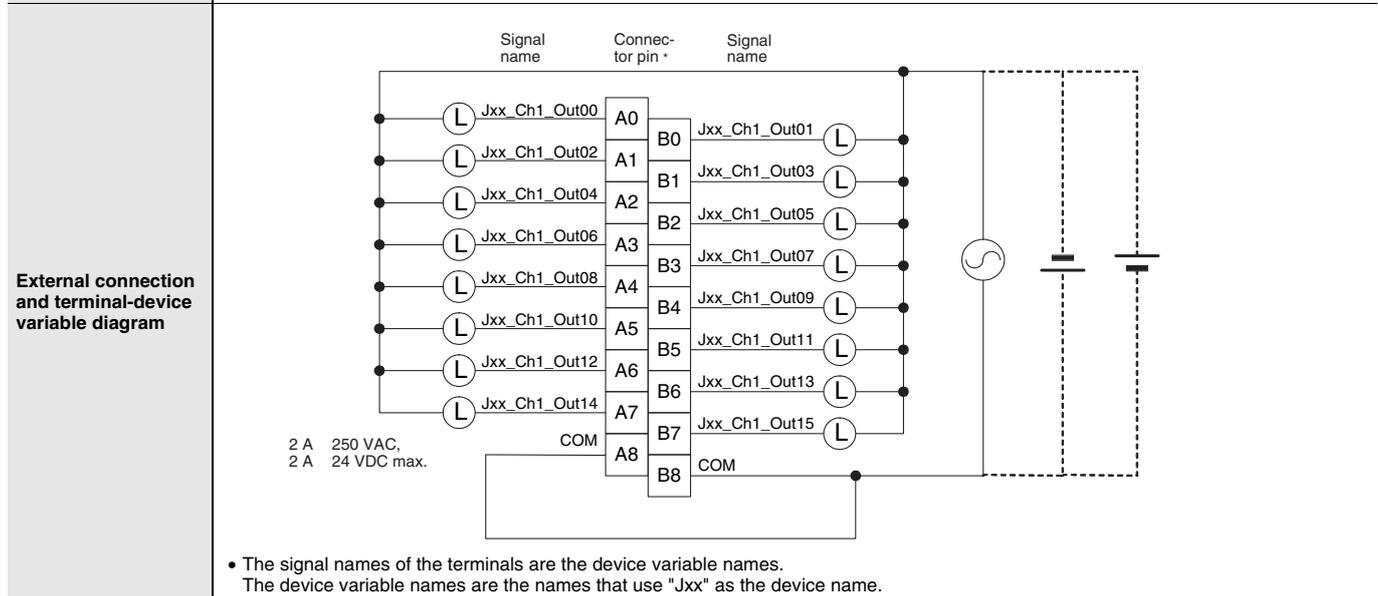
\* Terminal numbers A0 to A8 and B0 to B8 are used in the external connection and terminal-device variable diagrams. They are not printed on the Units.
