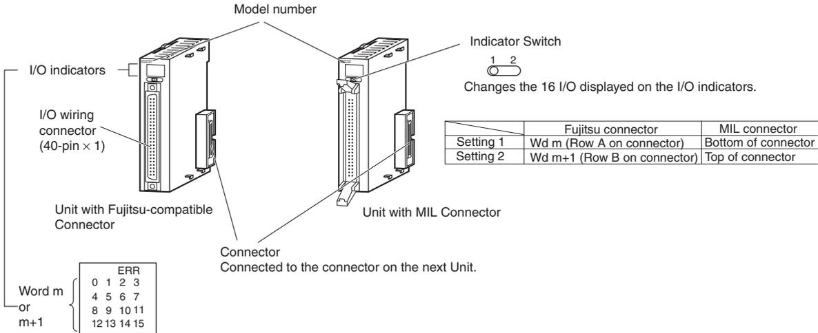
**Note:** Only the CJ1W-OD232 has an ERR indicator for the load short-circuit alarm.
