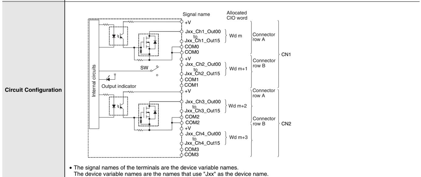
External connection and terminal-device variable diagram
