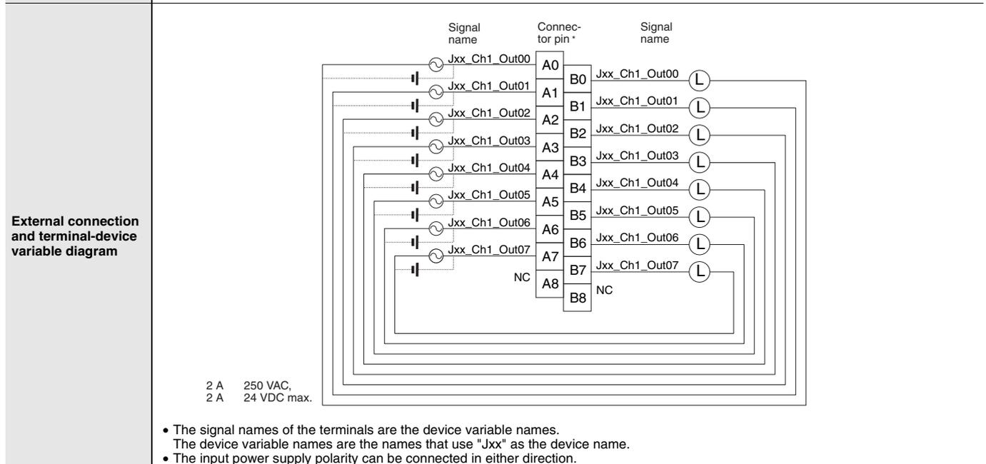
\* Terminal numbers A0 to A8 and B0 to B8 are used in the external connection and terminal-device variable diagrams. They are not printed on the Units.
