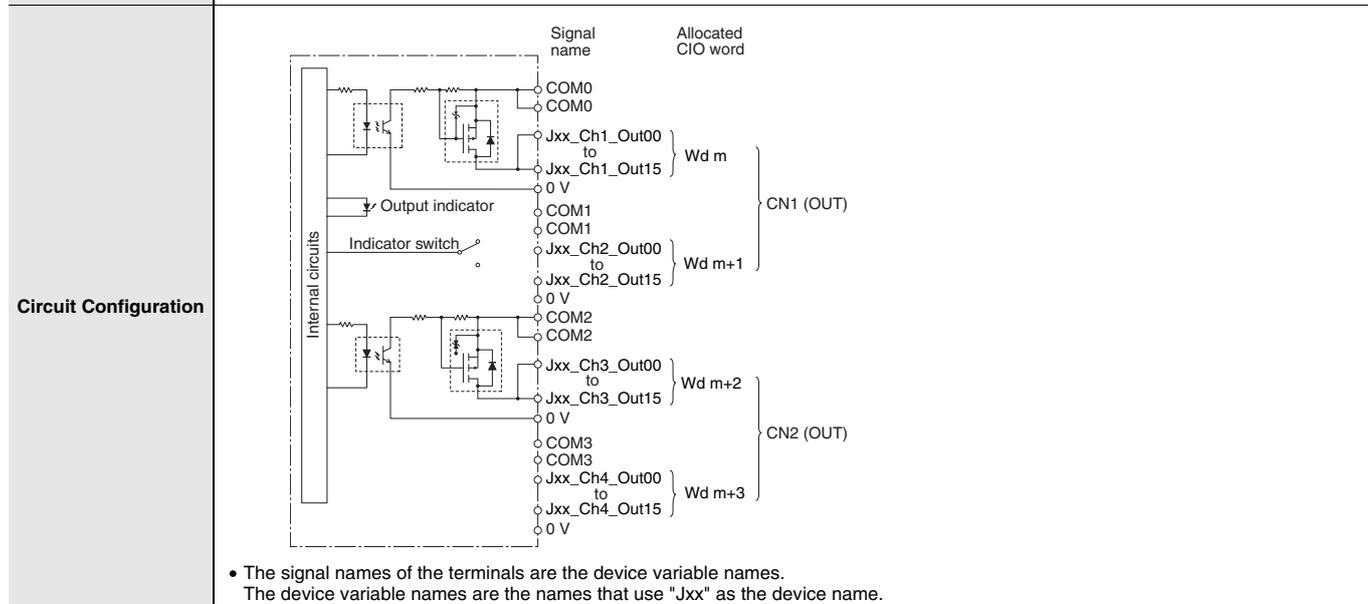
External connection and terminal-device variable diagram
