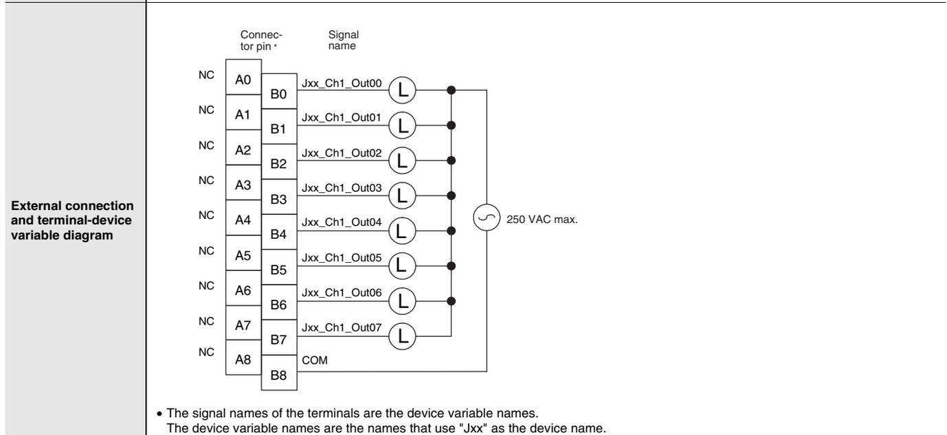
\* Terminal numbers A0 to A8 and B0 to B8 are used in the external connection and terminal-device variable diagrams. They are not printed on the Units.
