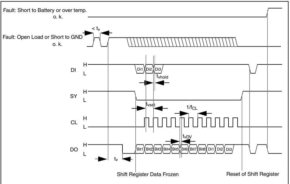
Figure 2. Serial Interface Error Coding
