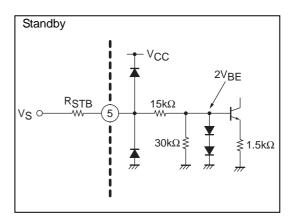
Note that the standby pin (pin 5) incorporates the anti-electrostatic diode, allowing the cu orrent to flow through the diode when the potential of  $V_{CC}$  pin 7 decreases below that of pin 5.
