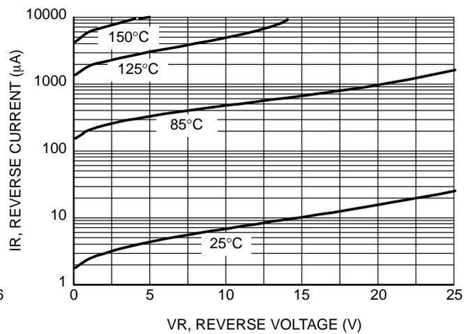
Figure 2. Leakage Current
