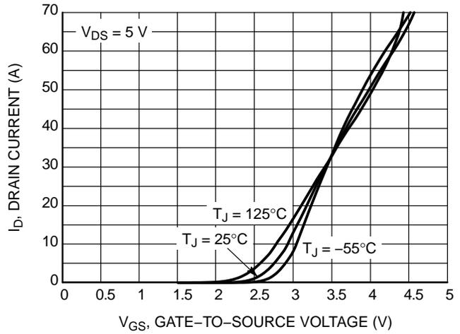
Figure 2. Transfer Characteristics
