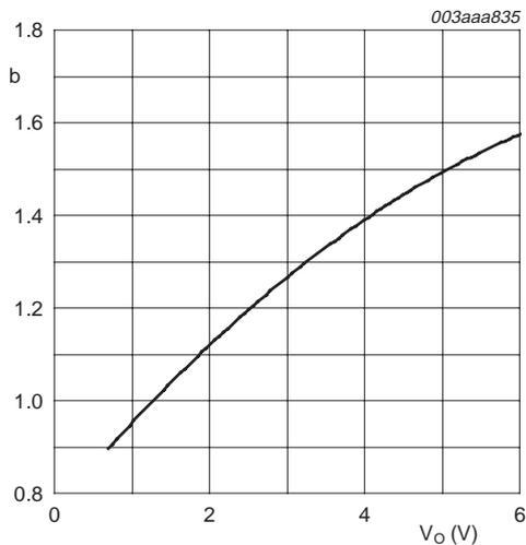
$V_{DDC} = 12\text{ V}; V_{DDO} = 12\text{ V}; f_i = 1\text{ MHz}; I_{O(AV)} = 25\text{ A}; V_{DDG} = 5\text{ V}$
