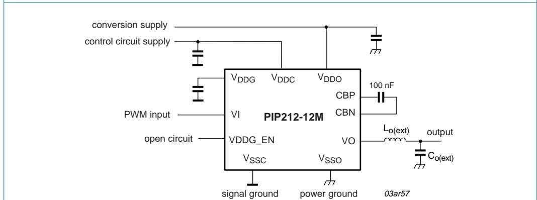
Fig 12. Single supply operation using internal supply for V<sub>DDG</sub>
