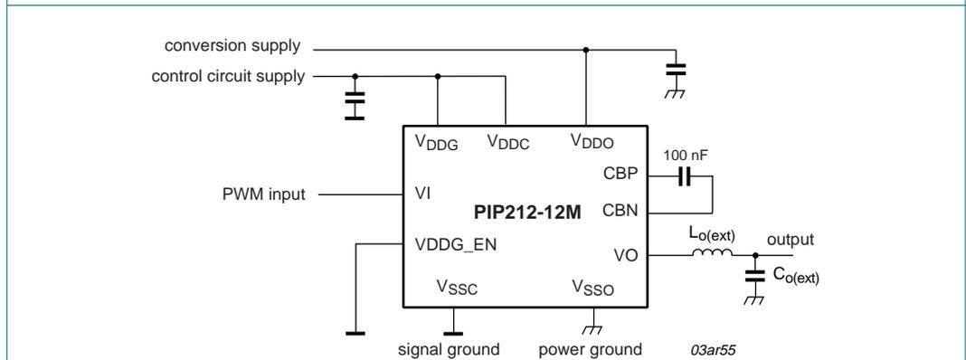
Fig 13. Single supply operation using external supply for V<sub>DDG</sub>
