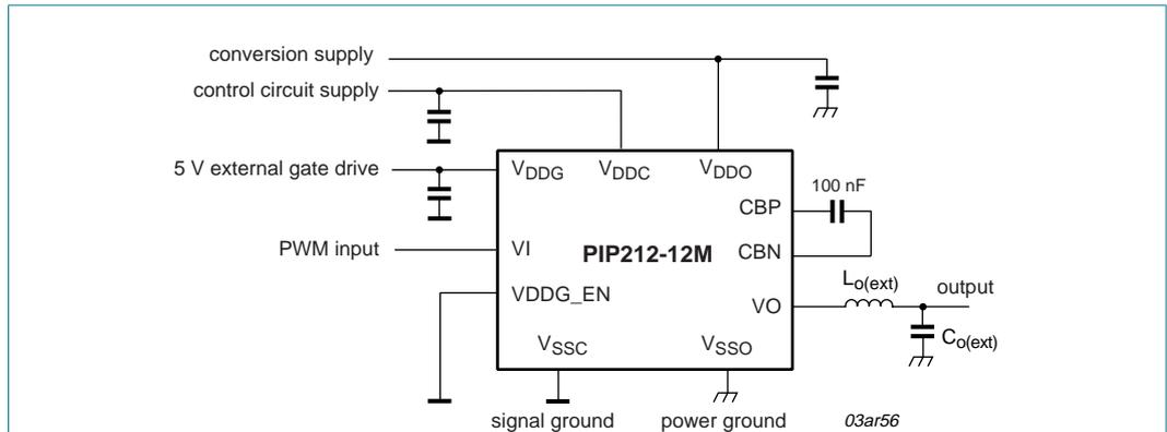
Fig 11. Dual supply operation using 5 V external supply for V<sub>DDG</sub>
