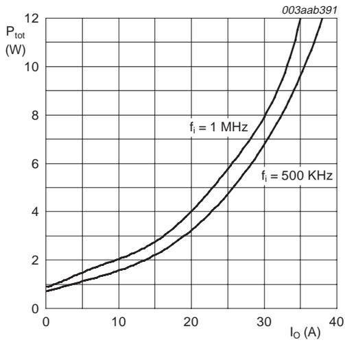
$V_{DDC} = 12\text{ V}; V_{DDO} = 12\text{ V}; V_O = 1.3\text{ V}; V_{DDG} = 5\text{ V}$
