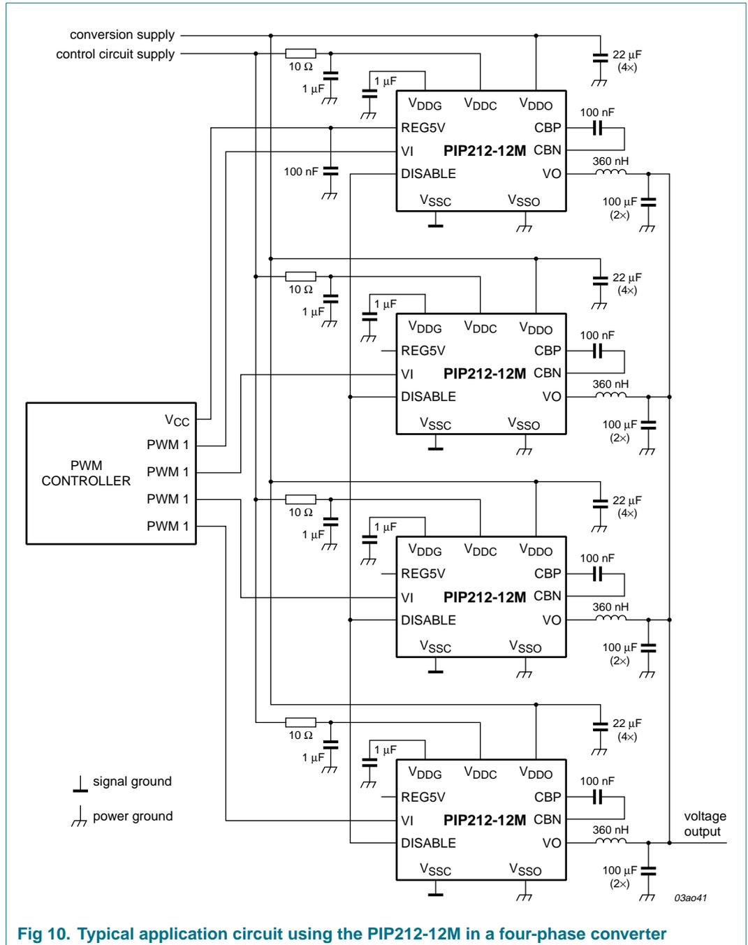
Fig 10. Typical application circuit using the PIP212-12M in a four-phase converter
