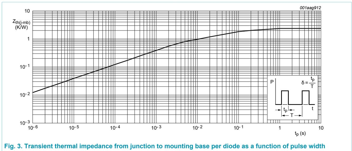
Fig. 3. Transient thermal impedance from junction to mounting base per diode as a function of pulse width
