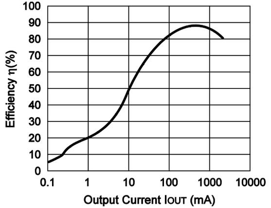
R1225N182D ( $V_{IN}=5.0V$ ) CDRH127-10 $\mu$ H
