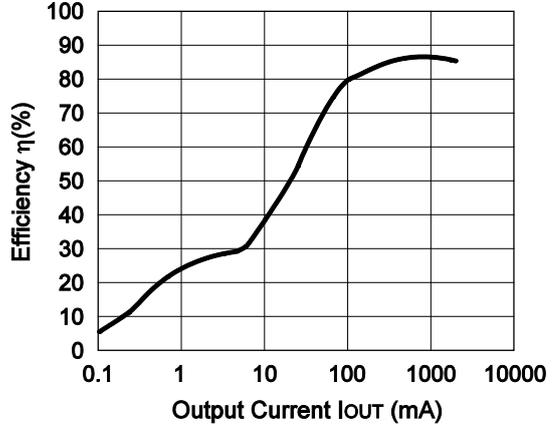
R1225N182C ( $V_{IN}=12V$ ) CDRH127-10 $\mu$ H
