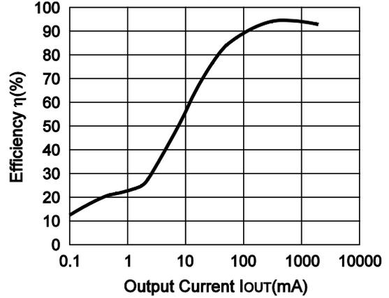
R1225N332C ( $V_{IN}=12V$ ) CDRH127-10 $\mu$ H
