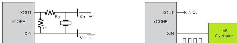
$R_f$  should be  $1\text{M}\Omega$ . Values for  $C_{11}$ ,  $C_{12}$  and  $R_d$  depend on the crystal characteristics. We recommend that you use a crystal with characteristics as specified in Table 11. These have an ESR of at most  $60\ \Omega$ , have a load capacitance of  $12\ \text{pF}$ , and all resonate at their fundamental frequency.
