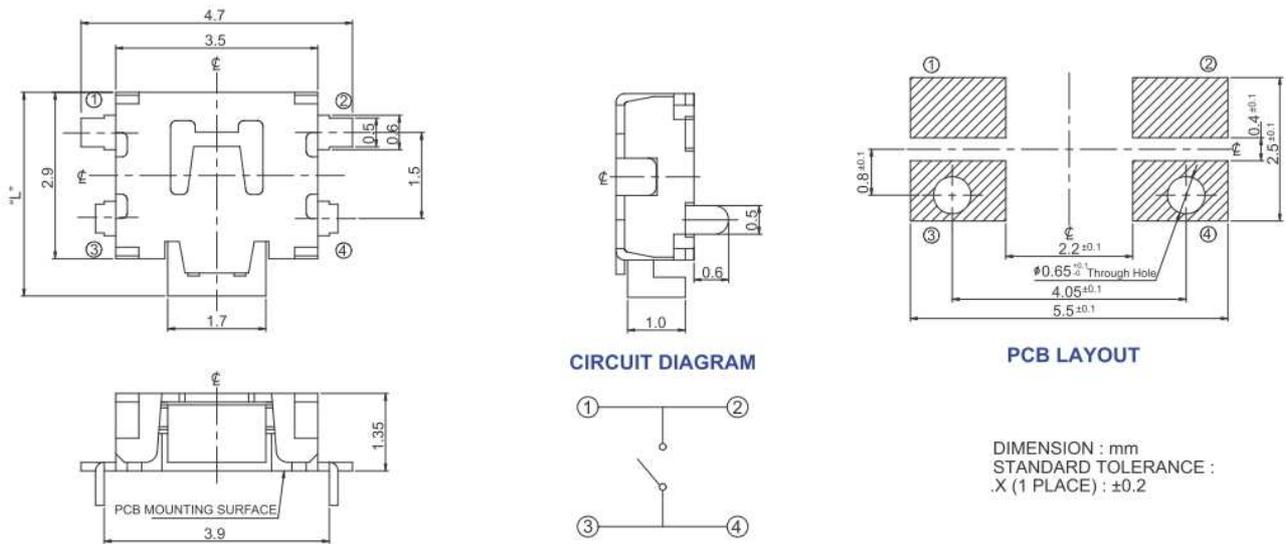
Figure 3 – 226EM1...(B)G, Surface Mount Gull Wing Type 1, With Ground Terminal
