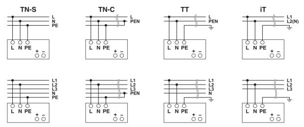
The connection for 100 V AC ... 240 V AC is established using the L, N, and P screw connections.
