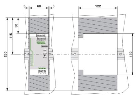
Slim-style installation: Installation depth 125 mm (+ DIN rail) (state at delivery)
