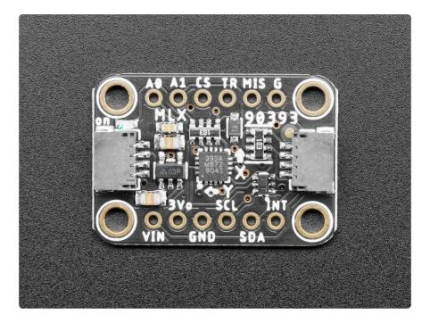
Measure the invisible magnetic fields that surround us, with this wide-range magnetometer. The MLX90393 is a wide range magnetic field sensor, that can measure 16-bits in ranges from  $\pm$ -5mT up to  $\pm$ -50mT in all 3 axes.
