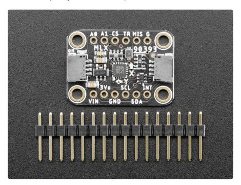
Comes as a fully assembled and tested breakout board with a small piece of header for use with a breadboard. As if that weren't enough, we've now also added <a href="SparkFun qwiic">SparkFun qwiic</a> () compatible <a href="STEMMA QT">STEMMA QT</a> () connectors for the I2C bus so you don't even need to solder the I2C and power lines. Just wire up to your favorite micro using a <a href="STEMMA">STEMMA</a> QT adapter cable. () The Stemma QT connectors also mean the MLX90393 can be
