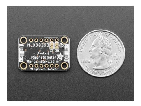
To make it easy to use, we've placed this tiny little sensor onto a breakout board, with a 3.3V power supply and level shifter. This makes it easy to use with any 3 or 5V microcontroller. Our Arduino and CircuitPython code will get you started in a jiffy, with I2C communication to the sensor. You will be readin' out those Gauss's in minutes! With the address select pins you can have up to 4 sensors on one I2C bus.
