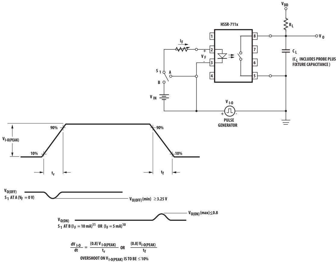
**Figure 19 Voltage Offset Test Setup**
