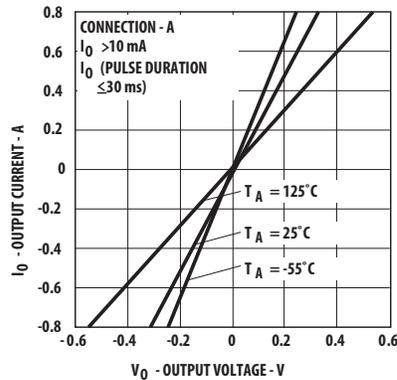
Figure 8 Typical Output Leakage Current vs. Temperature
