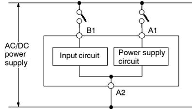
Since the input circuit and the power supply circuit are configured independently, the input circuit can be turned on or off irrespective of the on/off state of the power supply. It must be noted that a voltage equivalent to the power supply voltage is applied to the input circuit.
