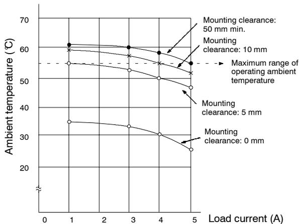
Note: Measurement Condition: Input voltage of 230 VAC.
