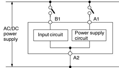
Since the input circuit and the power supply circuit are configured independently, the input circuit can be turned on or off irrespective of the on/off state of the power supply. Note that a voltage equivalent to the power supply voltage is applied to the input circuit.
