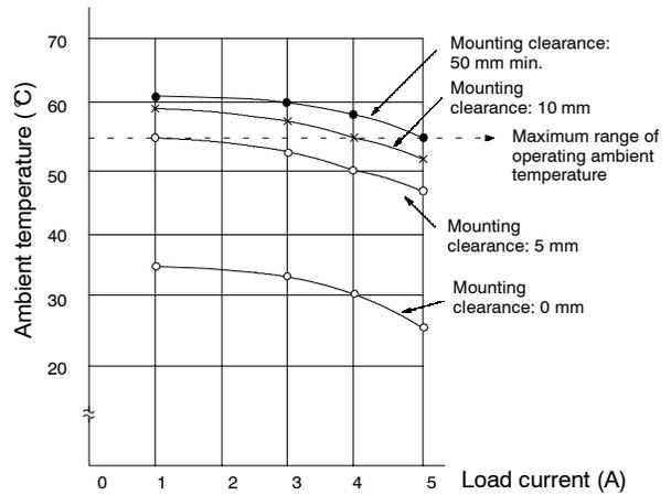
(Measurement Condition: Input voltage of 230 VAC)
