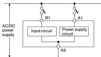
Since the input circuit and the power supply circuit are configured independently, the input circuit can be turned on or off irrespective of the on/off state of the power supply.
