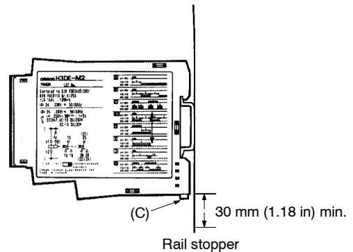
The H3DE can be mounted or removed easily if a distance of 30 mm (1.18 in) or more is kept between the H3DE and the top surface of other equipment located below the H3DE.
