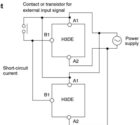
The H3DE Series is provided with a transformerless power supply system.
