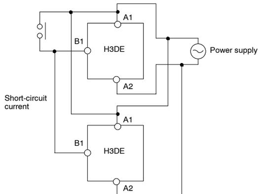
**Note:** The H3DE Series is provided with a transformerless power supply system.
