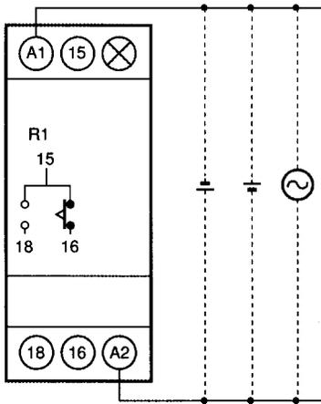
Note: DC supply voltage does not require the designation of polarity.
