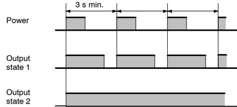
If it is required that the output be turned on repeatedly with an interval of shorter than 3 s, consider use of the H3DE-M2/-M1 in mode D (signal OFF-delay).
