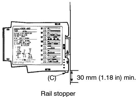
The H3DE can be mounted and removed easily if a distance of 30 mm (1.18 in) or more is kept between the H3DE and the top surface of other equipment located below the H3DE.
