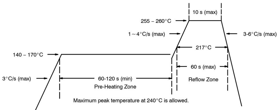
FIGURE 3. Solder Reflow Temperature and Time Durations
