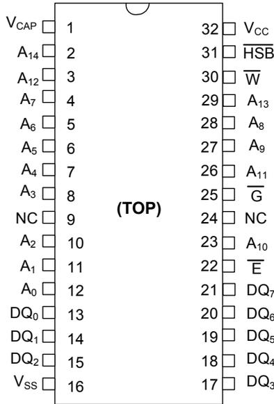
Figure 2. Pin Diagram - 32-Pin 450 Mil LCC
