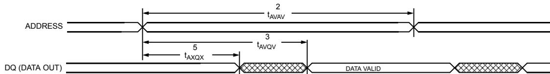
**Figure 5. SRAM Read Cycle 2:  $\bar{E}$  and  $\bar{G}$  Controlled** <sup>[6]</sup>
