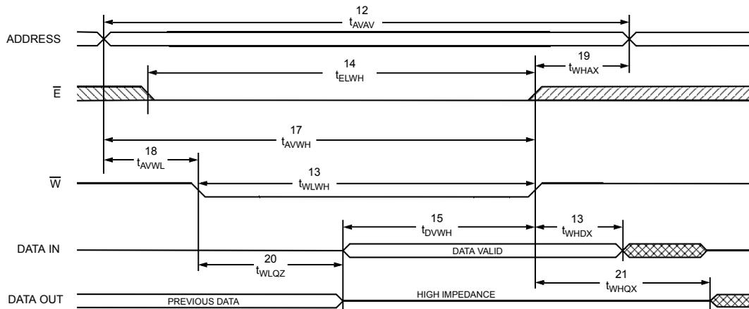
Figure 7. SRAM Write Cycle 2:  $\bar{E}$  Controlled [13, 14]
