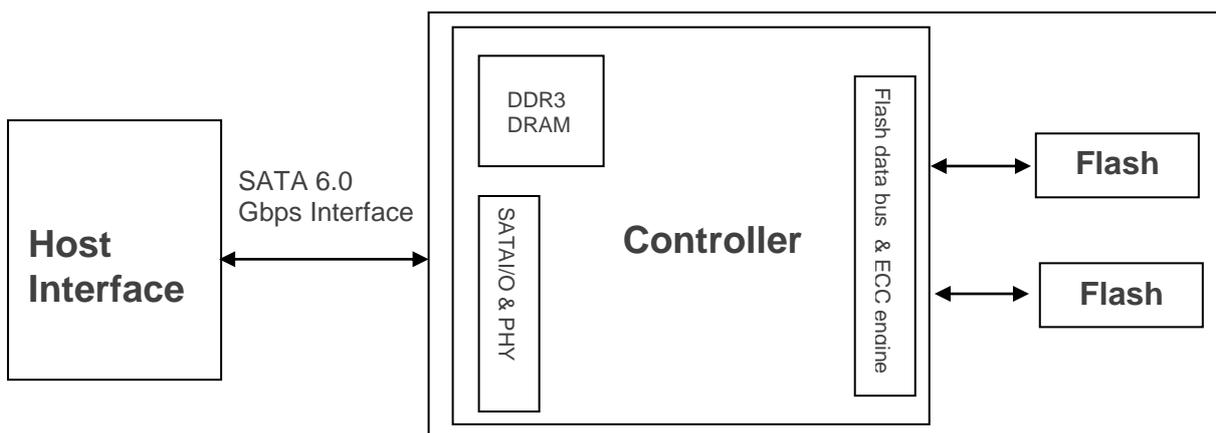
Figure 2-1 Block Diagram
