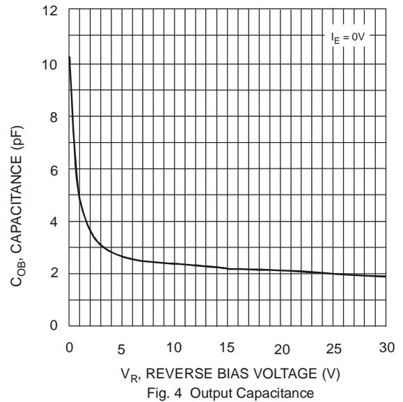
Fig. 4 Output Capacitance
