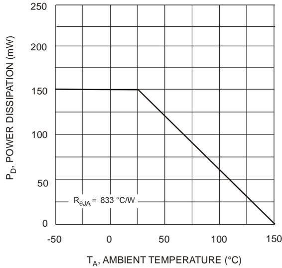
Fig. 1 Derating Curve
