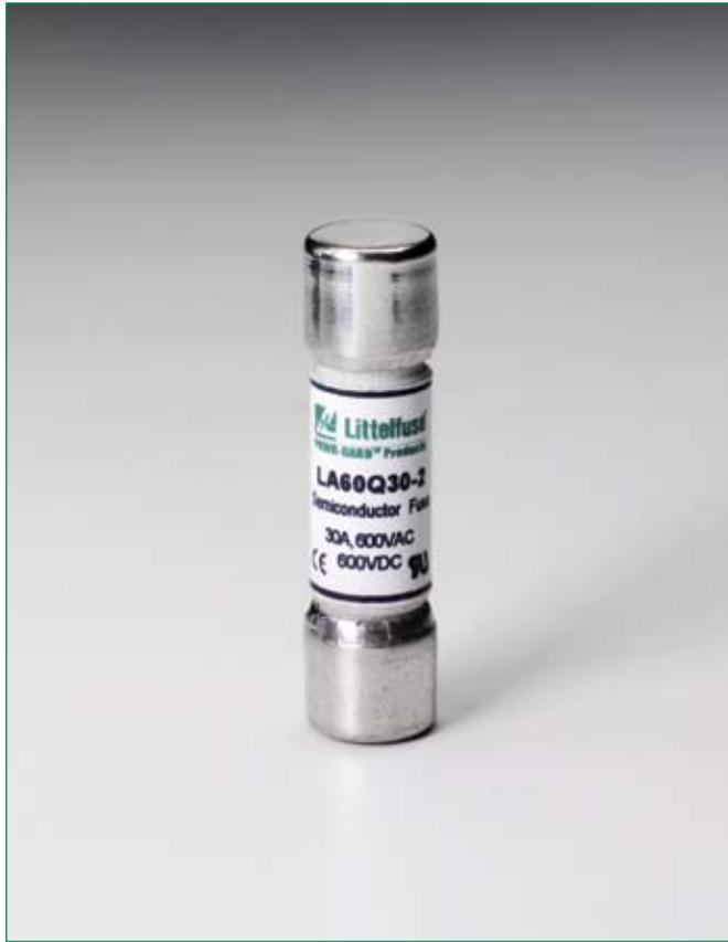
Littelfuse LA60Q semiconductor protection fuses feature a 600 volt AC/DC rating in a compact size (1½" x 13/32"). LA60Q also has the lowest I<sup>2</sup>t of all similar fuses and excellent cycling ability. Applications include inverters and small equipment requiring extremely fast response to faults, without the need to carry sustained heavy overloads.
