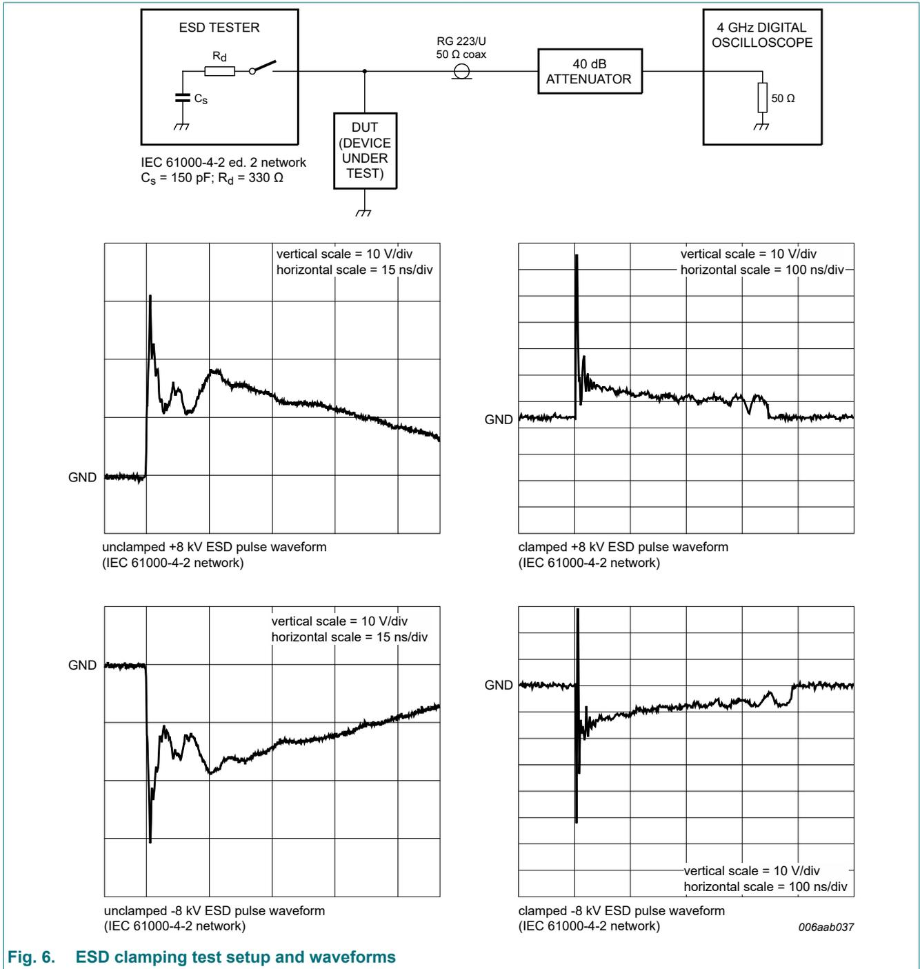
Fig. 6. ESD clamping test setup and waveforms
