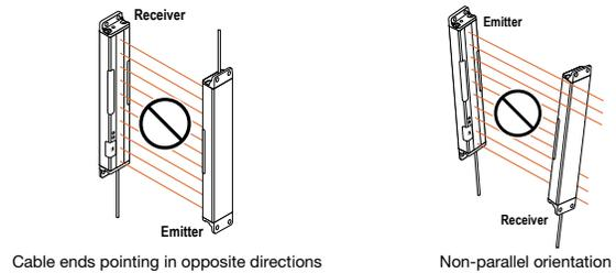
Figure 3. Maximum Off-Axis Misalignment
