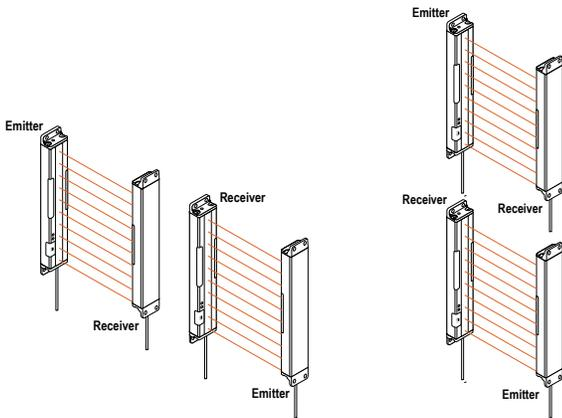
Figure 2. Example—Incorrect Positions
