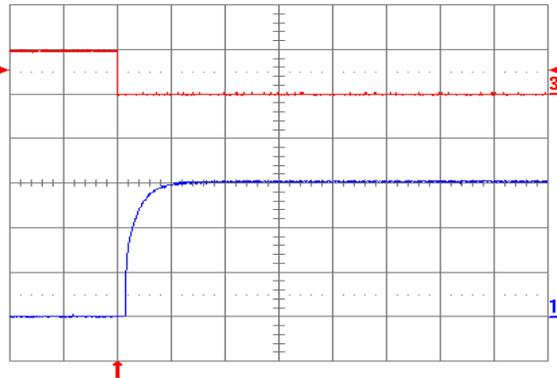
Fig. 7: Turn-on transient at full rated load current (resistive) with no output capacitor at  $V_{in} = 48\text{ V}$ , triggered via ON/OFF pin. Top trace: ON/OFF signal (5 V/div.). Bottom trace: output voltage (2 V/div.). Time scale: 5 ms/div.
