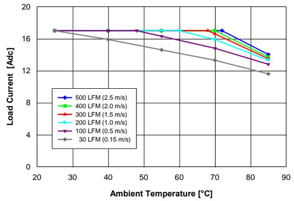
Fig. 2: Available load current vs. ambient air temperature and airflow rates for converter with G height pins mounted horizontally with air flowing from pin 1 to pin 3 and maximum FET temperature  $\leq 120\text{ }^{\circ}\text{C}$ ,  $V_{in} = 48\text{ V}$ .
