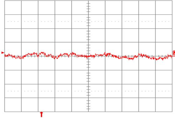
Fig. 14: Input reflected ripple current,  $i_s$  (10 mA/div.), measured through 10  $\mu$ H at the source at full rated load current and  $V_{in} = 48$  V. Refer to Fig. 12 for test setup. Time scale: 1  $\mu$ s/div.
