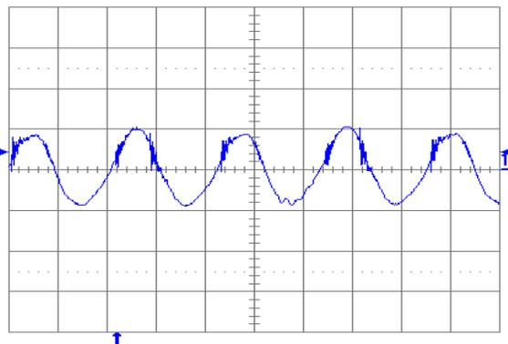
Fig. 11: Output voltage ripple (20 mV/div.) at full rated load current into a resistive load with  $C_o = 10\ \mu\text{F}$  tantalum + 1  $\mu\text{F}$  ceramic and  $V_{in} = 48\text{ V}$ . Time scale: 1  $\mu\text{s}$ /div.
