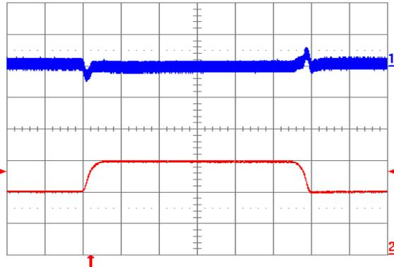
Fig. 9: Output voltage response to load current step-change (10 A – 15 A – 10 A) at  $V_{in} = 48\text{ V}$ . Top trace: output voltage (100 mV/div.). Bottom trace: load current (5 A/div.). Current slew rate: 0.1 A/ $\mu\text{s}$ .  $C_o = 1\ \mu\text{F}$  ceramic. Time scale: 0.2 ms/div.
