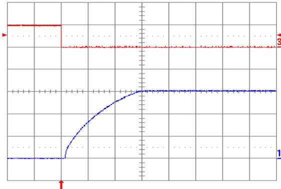
Fig. 8: Turn-on transient at full rated load current (resistive) plus 10,000  $\mu\text{F}$  at  $V_{in} = 48\text{ V}$ , triggered via ON/OFF pin. Top trace: ON/OFF signal (5 V/div.). Bottom trace: output voltage (2 V/div.). Time scale: 5 ms/div.
