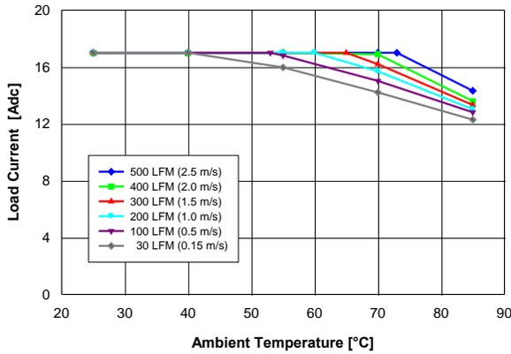
Fig. 1: Available load current vs. ambient air temperature and airflow rates for converter with G height pins mounted vertically with air flowing from pin 1 to pin 3 and maximum FET temperature  $\leq 120\text{ }^{\circ}\text{C}$ ,  $V_{in} = 48\text{ V}$ .
