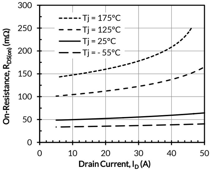
Figure 5. Typical drain-source on-resistances at  $V_{GS} = 12V$
