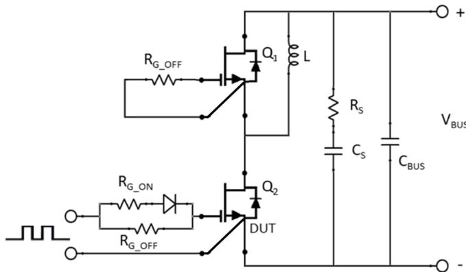
Figure 22. Schematic of the half-bridge mode switching test circuit. A bus RC snubber ( $R_S = 2.5\Omega$ ,  $C_S = 100nF$ ) is used to reduce the power loop high frequency oscillations.
