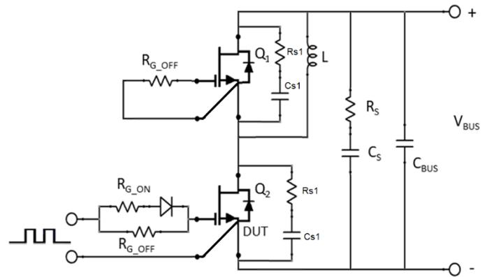
Figure 23. Schematic of the half-bridge mode switching test circuit with device RC snubbers ( $R_{s1} = 5\Omega$ ,  $C_{s1} = 95pF$ ) and a bus RC snubber ( $R_S = 2.5\Omega$ ,  $C_S = 100nF$ ).
