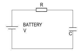
When a capacitor is connected to an item such as a battery, charge will flow from the battery into it. Therefore the capacitor will begin to fill up. The flow of water in the picture above left is the equivalent of how the electrical charge will flow in the circuit shown on the right.
