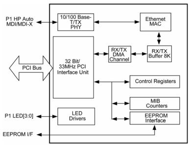
Figure 1. KSZ8841-PMQL Function Diagram
