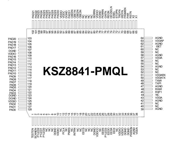
Figure 2. KSZ8841-PMQL 128-Pin PQFP (Top View)
