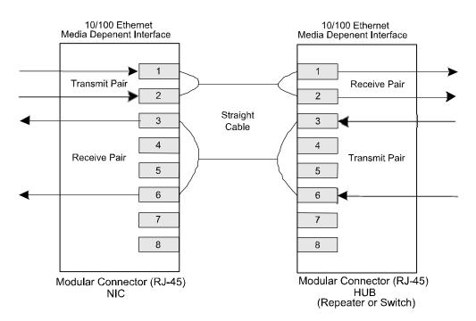
Figure 3. Typical Straight Cable Connection
