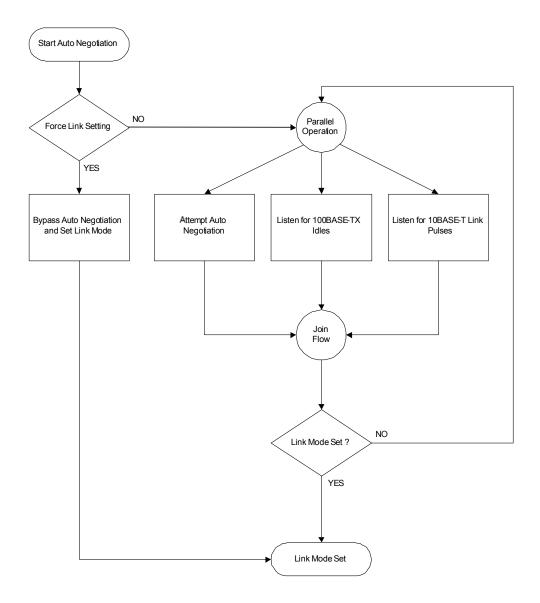
Figure 5. Auto Negotiation and Parallel Operation
