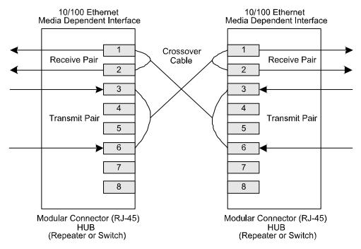
Figure 4. Typical Crossover Cable Connection
