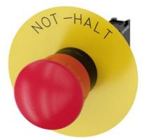
EMERGENCY STOP mushroom-type actuator, 22 mm, round, plastic, red, 40 mm, positive latching, according to EN ISO 13850, rotate-to-unlatch, with yellow backing plate, inscription: NOT-HALT, with holder, 1 NC, screw terminal, Z=20-unit packaging
