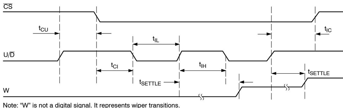
Figure 7. Serial Interface Timing Diagram, Increment Mode
