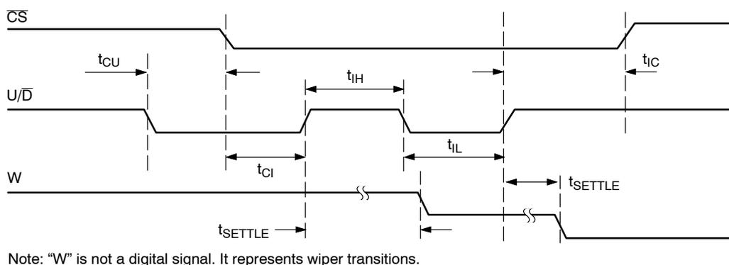
Figure 8. Serial Interface Timing Diagram, Decrement Mode
