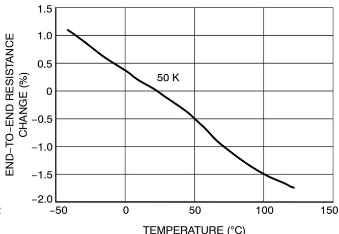
Figure 3. Change in End-to-End Resistance vs. Temperature
