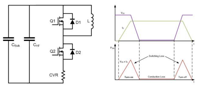
Figure 2. CIL Test Fixture Used to Measure the Switching Loss of MOSFET Q2
