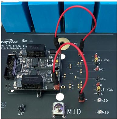
Figure 13. Dual-Channel Gate Driver with DESAT Cable Connections
