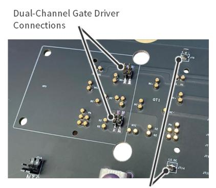
DESAT Connections Figure 12. Dual-Channel Isolated Gate Drive Interface
