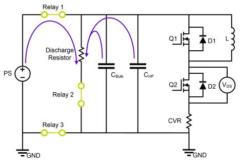
Figure 11. CIL test Fixture Schematic During the DISCHARGE State
