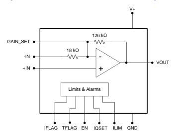
Figure 1. OPA521 Device Functional Block Diagram
