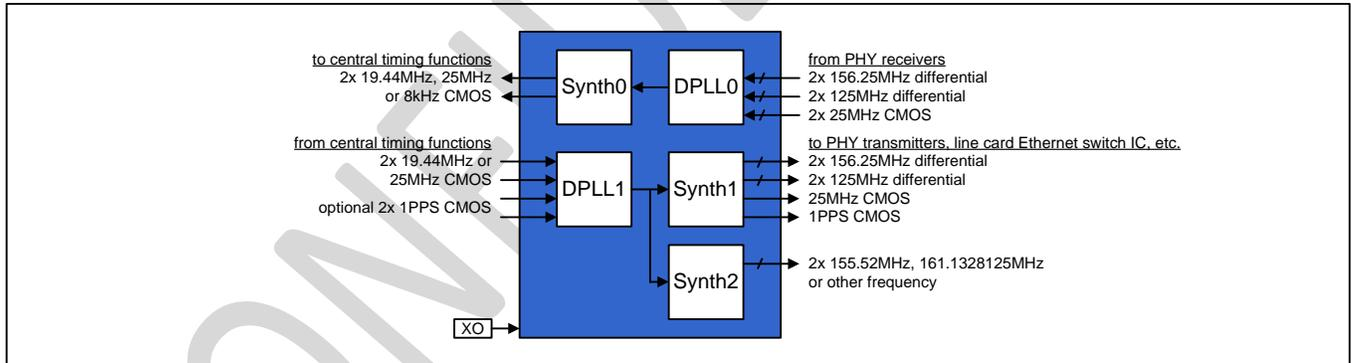
Figure 2 - Synchronous Ethernet and IEEE 1588 Line Card Application
