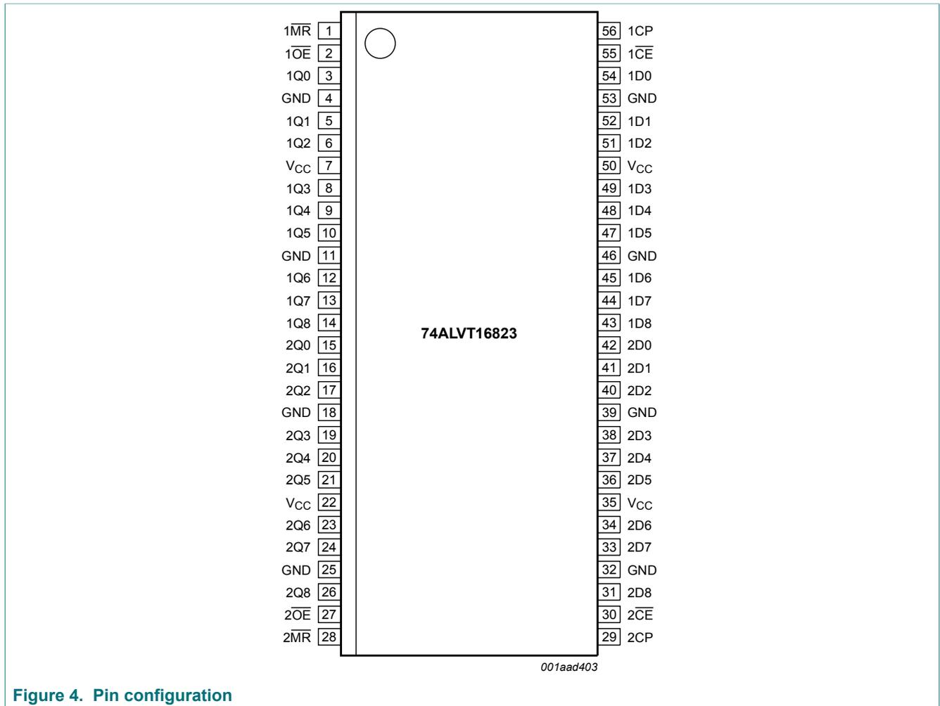
Figure 4. Pin configuration
