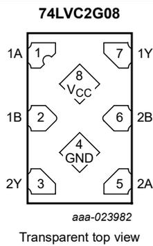
Fig. 6. Pin configuration SOT1233-2 (X2SON8)
